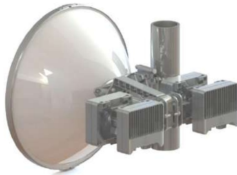
Figure 3 Dual polarized antenna equipped with two IPS3 and four MINI-LINK 6363
